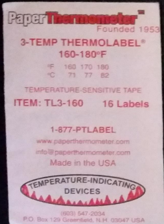
Strips to indicate hot water temperature sanitizing in dishmachines
